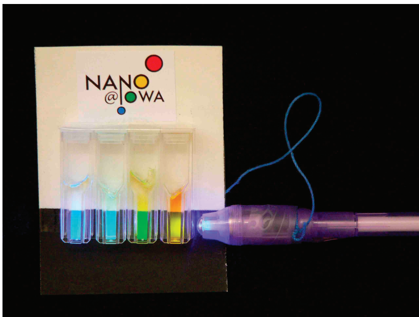
Figure 7.2. Cadmium selenide (CdSe) quantum dot samples embedded in a polymer are used for outreach activities. The luminescent properties can be observed using the attached violet LED pen lights. The NANO@IOWA logo on the cards reinforces the idea that the colors of the quantum dots depend on their size.
