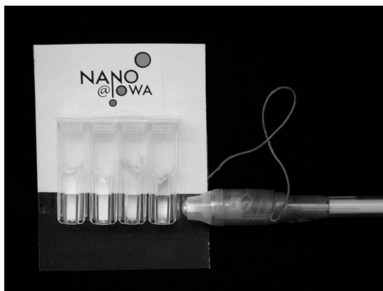
Figure 2. Cadmium selenide (CdSe) quantum dot samples embedded in a polymer are used for outreach activities. The luminescent properties can be observed using the attached violet LED pen lights. The NANO@IOWA logo on the cards reinforces the idea that the colors of the quantum dots depend on their size. (See page 3 of color inserts.)
